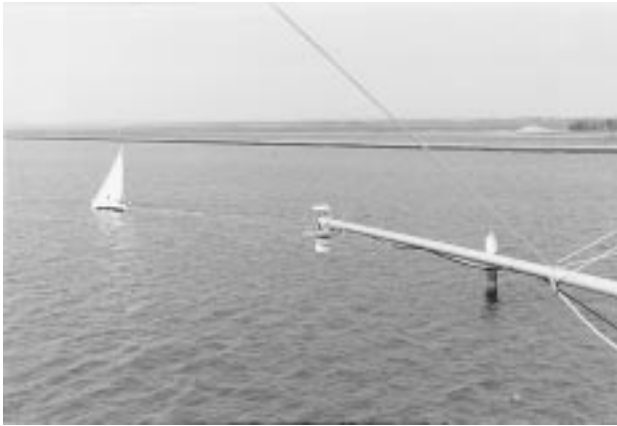
Fig. 2. Antenna arrangement: a RHCP 2-dBic zenith-looking and a LHCP 9-dBic nadir-looking antenna, back to back, at the tip of a 4.5 m mast over the edge of the bridge.
